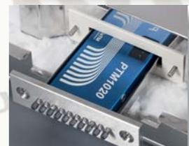
Stainless steel fittings protect against water and provide stress relief for the thermocouples.
