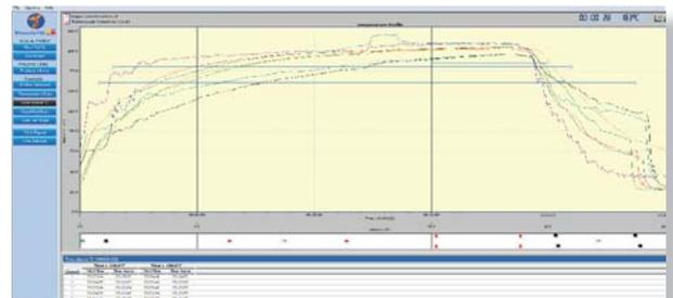
Multiple time above temperature, rates of change of temperature and maximum temperature analysis options for verification of the cure quality and optimisation of the process
